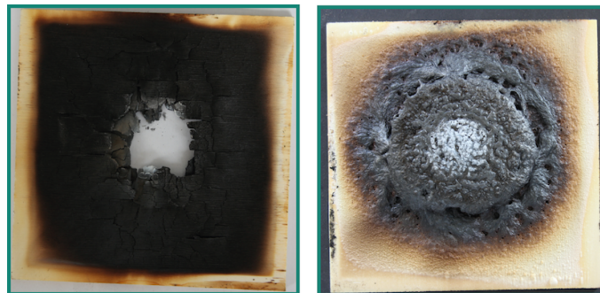
Figure 1: Results of Fraunhofer WKI's own fire test on untreated plywood (left, test time = 3 min.) and plywood with an intumescent coating (right, test time = 13 min.).
