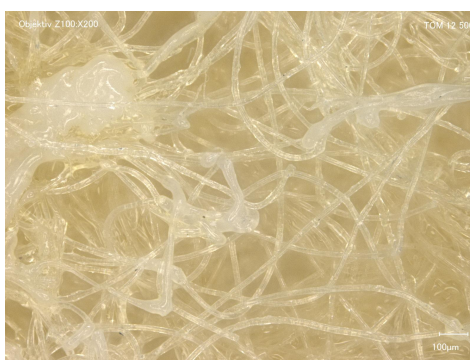
Figure 1: Textile with immobilized lipase.
