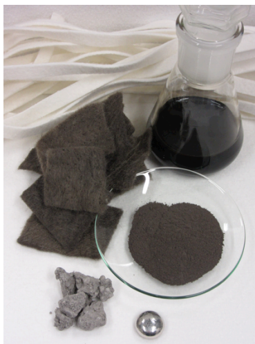
Figure 1: Different stages of precious metal recovery with polyelectrolyte-finished textiles.
